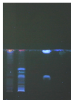
Fig. 1. Chromatogram obtained before revelation (mobile phase A) 1. TRFF ; 2. M-fr 3. rutin, hyperoside, isoquercitrin (bottom-up); 4. chlorogenic acid, caffeic acid (bottom-up); 5. ferulic acid.
